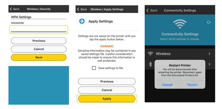
You have now successfully set up DHCP Connection on your printer. DHCP Connection will automatically assign a temporary, unused IP Address on your internet server to your printer. By finding out what this IP Address number is, we can then configure the printer to permanently be assigned that IP address. Once it is permanently assigned you will be able to use the printer through WiFi on your computer or another device connected to the same network.
