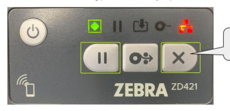
Hold down the outer two buttons until the printer starts feeding out blank labels
