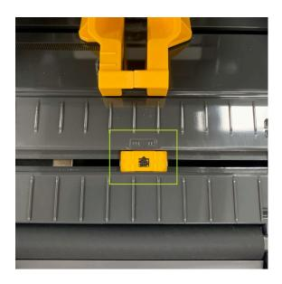
Ensure the arrow on the label sensor and the arrow marked into the plastic are aligned pointing towards each other.
